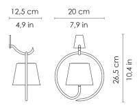
A rechargeable wall lamp with a matt white or corten painted aluminium fixture, a polycarbonate diffuser and a LED light source. Battery life guaranteed for more than 9 hours. Power charger with micro USB plug - included
